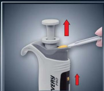
Remove the colour cap using the calibration key. Set the calibration switch in its upper position.
