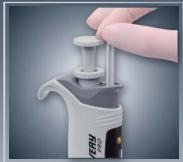
Insert the calibration key into the ejector orifice. Turn the key so as the volume indicated by the counter is equal to the average calculated volume.
